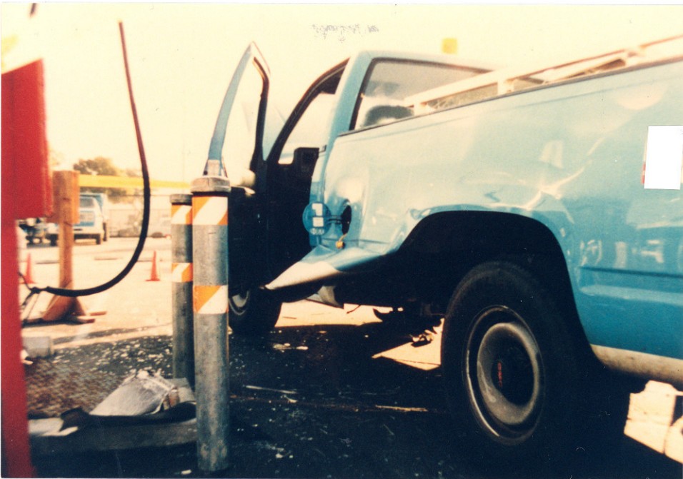
2. Left Side Damage to the CNG Truck Body and Debris
